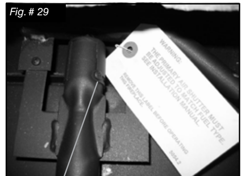
PRIMARY AIR SHUTTER (Shown in closed position for NG) (Fully open shutter for Propane)
