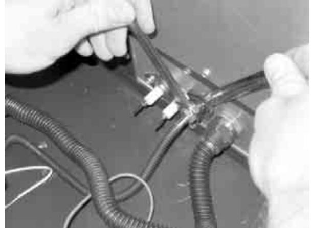
ATTACH PILOT SUPPLY TUBE
