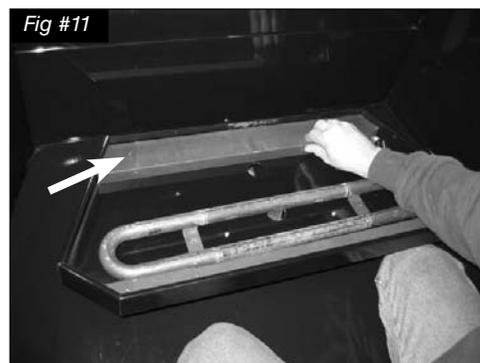
**Set the air shutter to fully open for Propane or fully closed for Natural gas.**
