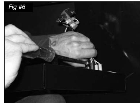
NOTE: Start screws with fingers first to prevent cross-threading.
